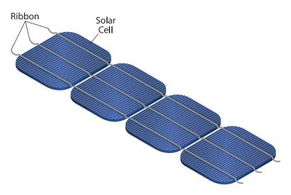
Solar cells are connected together to form a string. Multiple strings are combined to form a photovoltaic panel.
